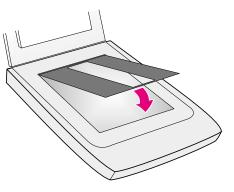
3 Slide up to three slides into the slide holder on the bottom side of the XPA light source. The correct view of the picture should be facing outward, toward you.
